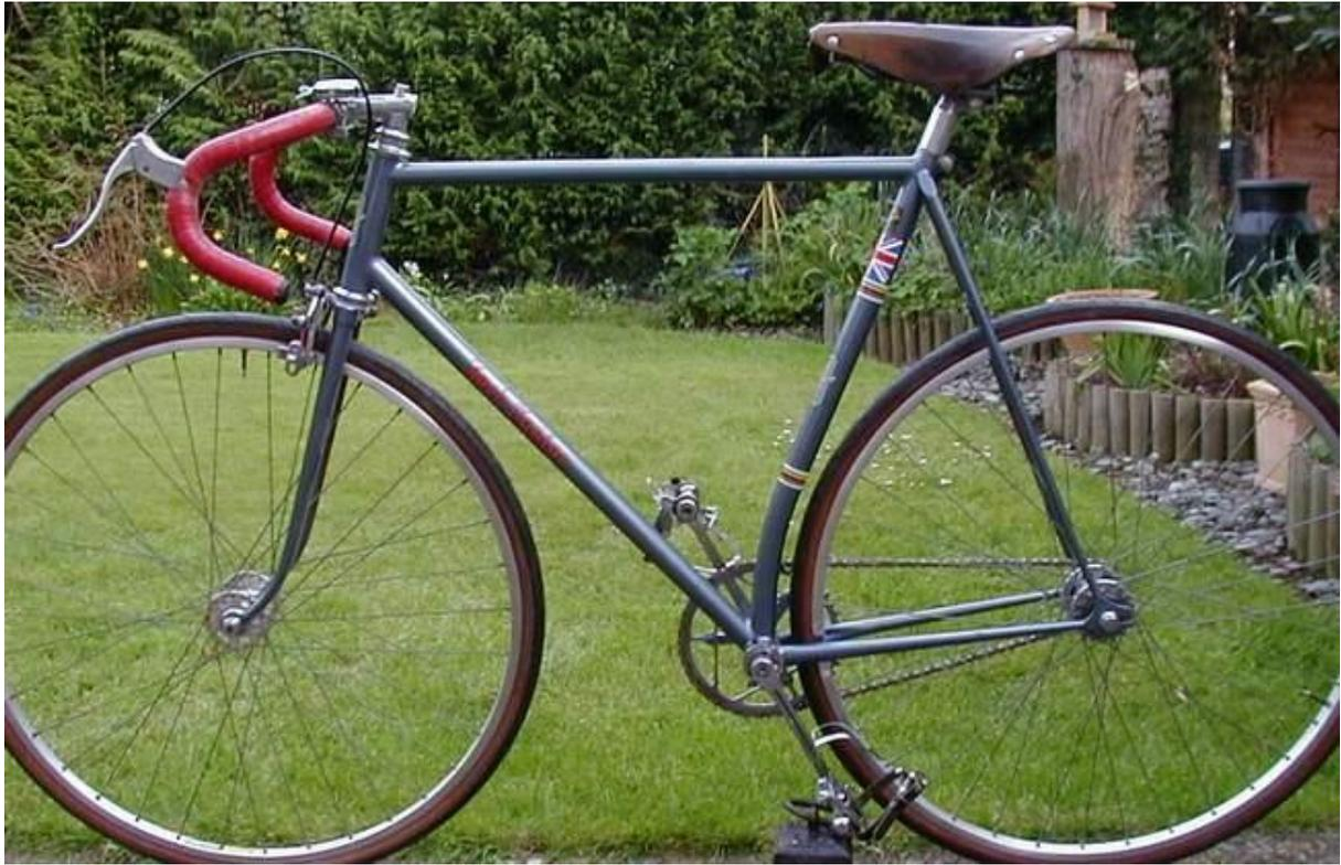
Many of these SWB machines had track ends although a few had forward-facing road ends. It is obvious that a frame built to tuck the rear wheel as far forward as possible would work better if the wheel could be taken out backwards rather than having to allow space for it to move forwards, the Jack Taylor above shows this in some detail. The advent of vertical rear dropouts obviated this problem of course.
