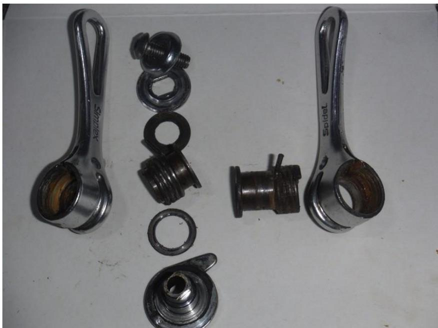
*LH lever assembly in pieces, plus a RH lever, drum and drag spring.*
